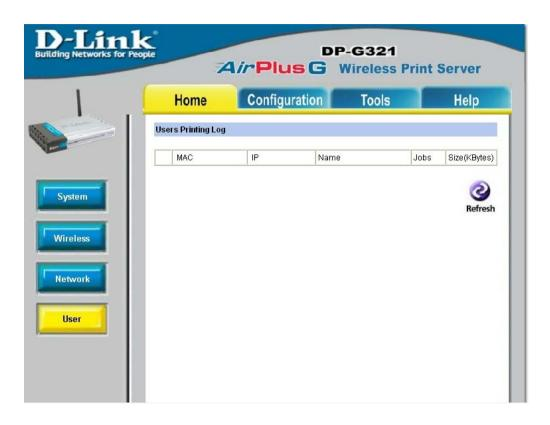
**Users Printing Log:** The items in this field display the user(s) information, which include the user(s) Mac address, IP address, name, and status of printing tasks.
